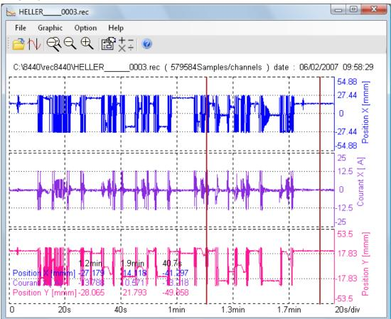
You can choose: Channels to be displayed The f(t) or XY mode Auto ranging of the channels
