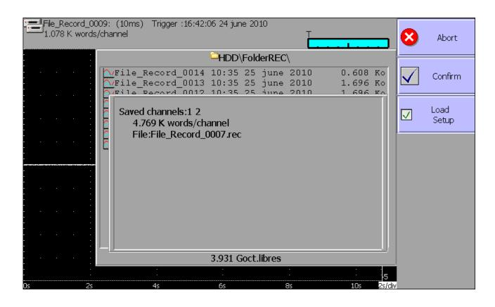
Select the place and the name of the file to load to display it on screen. You can recover the channels configuration (type, name, functions...) and the validations. For that you must validate "load configuration".
