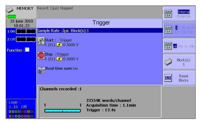
The programming of the triggers is different according to the current mode (Direct, Memory, GoNogo or File).
