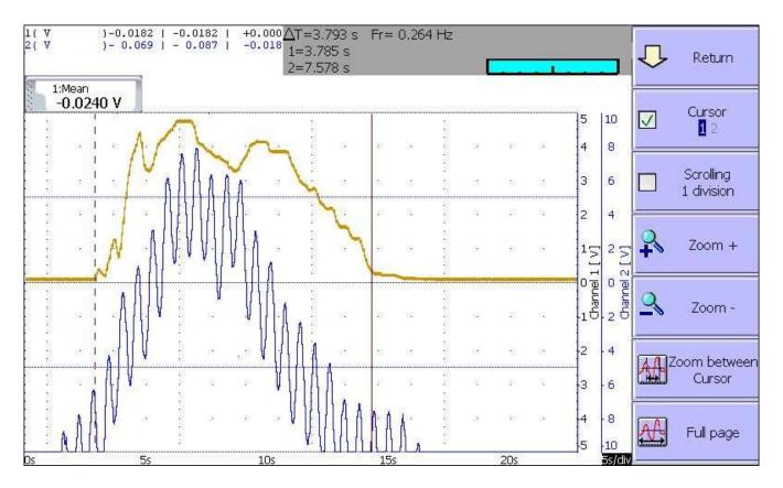
It is possible to trigger on a periodic signal parasite (50 Hz-main): the trigger is executed when the signal shape changes radically.
