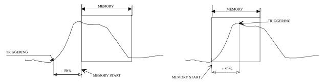
Transfer to memory with a -50% delay relatively to the beginning of the memory
